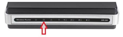
4. Wait for 30-60 seconds for the process to complete, once the Status LED is blinking and usually if an Ethernet connected computer is connected either Ports 1, 2, 3 or 4 will be illuminated again to advise the reset process has been completed.
